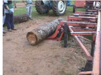
hydraulically powered lifting arms. The arms lift the log and position it on the frame. You'll notice that the Wood-Mizer only
