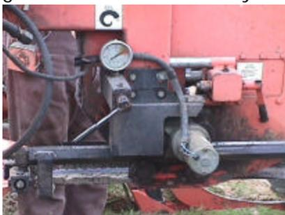
motors move the cutting head up and down, the cutting carriage forward and backward on the track and adjust the blade
