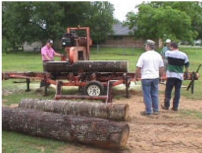
model LT40-HD can handle logs up to 21' long and 36" in diameter. It can cut boards as wide as 28" in one pass. Bill's
