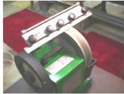
jig to hold the blades at a precise angle during the sharpening process. Tormex provides an angle gauge with their system that helps if you want to change the angle of
