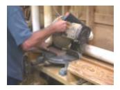
Now it's time to cut the pieces to length. Jerry believes that radial arm saws are only good to rough cut pieces to length. He uses a miter saw with a long support table to make
