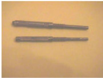
inside of the brass barrels. I prefer to use an adjustable reamer. Use a 1/4" to 9/32" reamer for 7mm
