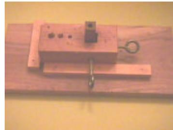
board – it MUST be square to the bottom of the jig. The holders are eyebolts in threaded inserts. You will also need a
