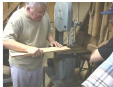
the sled as a guide and carefully cut each tail on the band saw. Finish cleaning up the tail with a chisel.
