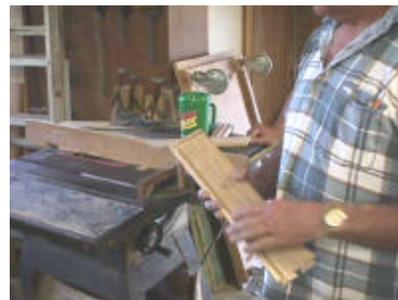
edge about 1/8" and routes the edge with a bullnose bit. Then he cuts the groove for the bottom in the front and side
