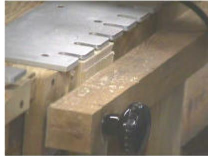
doing a shallow cut across the face of the board before you make the full cut for the tails and pins.
