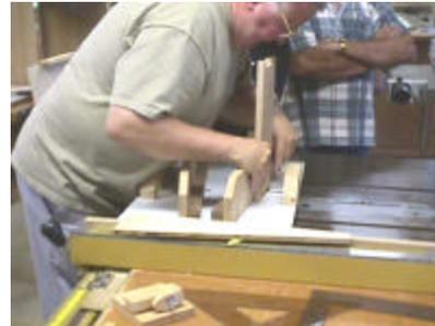
next pin and repeat the cut. When you've finished these cuts on all of the pin boards, turn the sled around and cut the
