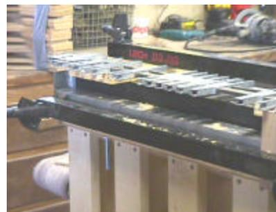
dovetails, John suggests the Leigh Jig. The fingers are adjustable and they're used cut the pins and the tails
