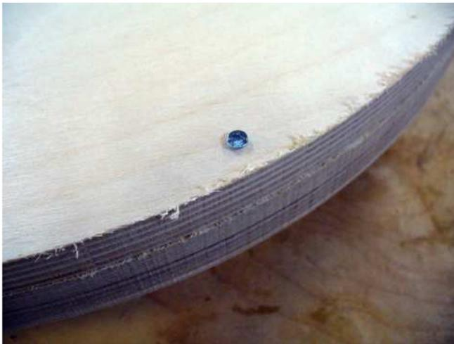
Next, I attached a faceplate to the center of one of the disks using screws that **just went only into this one!** The faceplate will be permanent so you need to get one specifically for the Longworth chuck.
