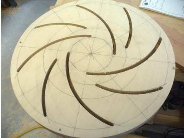
At this point I put it back on the lathe and with a 1/4" drill bit in a Jacob's chuck on the tailstock I drilled a hole completely through the center. I also drilled a couple of holes around the very outside edge so that I could use tommy bars to tighten.
