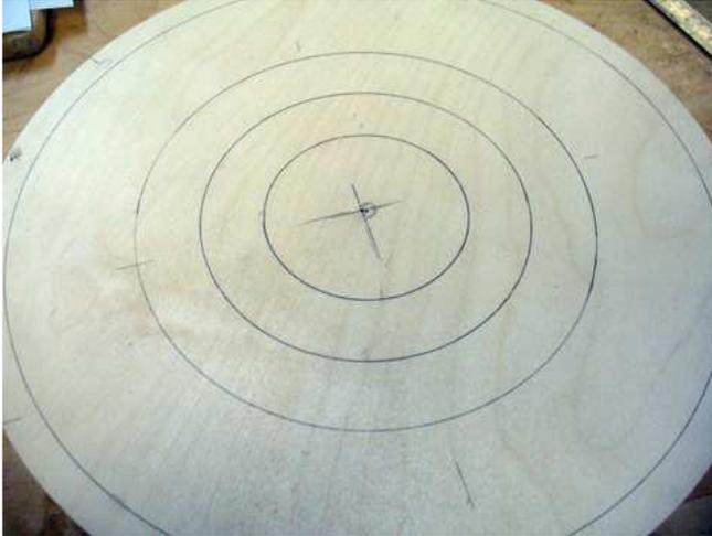
Next, using a ruler I drew a line across the diameter of the disk and then using a protractor I drew a line 90 degrees to this one. Then I drew 2 more lines at 45 degrees to the first one. This made 8 evenly spaced segments:
