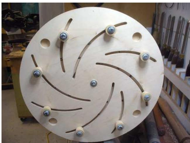
The Longworth chuck was developed in the late 1980's by Leslie Douglas Longworth of the Hunter Valley Woodturners in Australia. It features a self centering mechanism that easily and quickly adjusts to the size of your turning.
