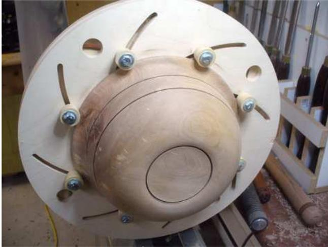
Because there are 4 arcs that don't come as close to the center as the other 4 there is a limit to how small of a piece you can fit on. The solution is to remove those 4 bolt assemblies and just use it with the 4 buttons on the larger arcs. This isn't a problem since a smaller piece will require less holding power. Another solution is to just make a smaller one with just 4 buttons. 😊
