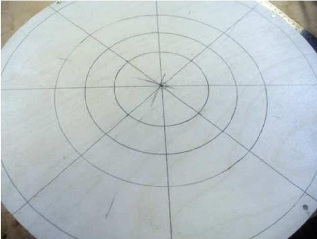
Then, with the point of a compass on the points where the second circle from the edge and the diameter lines intersect, I drew an arc tangent to the inner circle to a point where they reach the outer circle. This is probably the most confusing part of making a Longworth and is more simply done than read. Hopefully this photo will help:
