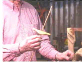
homemade gauge consisting of a crosshead with a hole, a dowel and a screw to tighten the crosshead to the dowel. Commercial versions are also available from woodworking catalogs.
