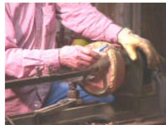
the bottom of the hole. Lyman uses the thin version of super glue around the edge of his natural edged bowls to keep the softer sap wood and bark firmly attached to the bowl during the turning process. The boring bar is a good alternative to a bowl gouge because
