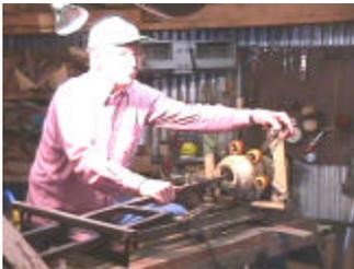
Lyman made his own boring bar from 1" square tubing. It's basically a large frame with a long bar on one side. A replaceable cutting tip (usually like a round nose scraper) is mounted on the end of the bar. A special steady rest keeps the bar from twisting and keeps it level while it's cutting. The result is a very stable cutting tool that you only have to guide when using.
