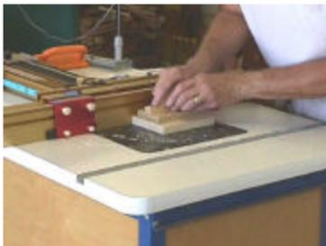
cut bit and a cutting depth of 1/16". Make the cross-cuts first, then rotate the blank and make the other cuts. The next pass uses a 3/8" bit set to 1/8" depth and the
