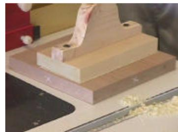
further away from the router bit. The fence stops are set so the cuts will stop 11/16" from the edge of the blank. Using the DOVG template, the spacing
