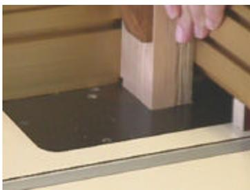
like maple or cherry) and marked one edge – this edge always stays against the fence. The pieces should be stacked together, along with a backing board, and cut at the
