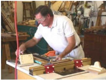
re-setting the fence many times. The Inkra-Jig 'sawtooth' alignment method provides a fast and easy way to make these repetitive adjustments.
