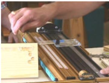
incorporates a micrometer that allows .001" adjustments. Gerald's set included the adjustable fence, stop blocks, height gauge, templates and project
