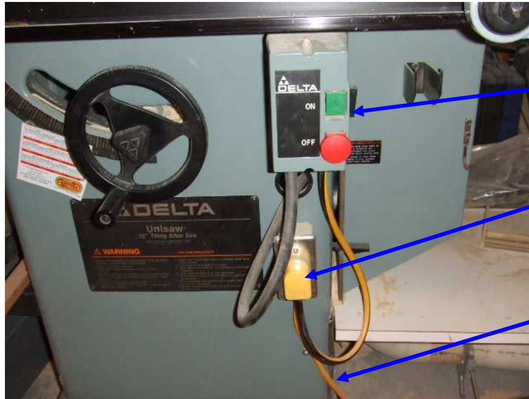
Delta Unisaw Electrical Connections
