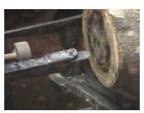
bars available, but Lyman built his own boring bar out of 1" square tubing, a piece of round stock and a piece of 1/8" by 3/4" tool steel.
