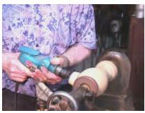
on a foam pad that's chucked in an electric drill. With the sanding disk spinning across the grain while the vase or bowl
