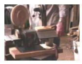
Lyman uses a grinder to establish the basic shape of his tool and then a combination disk/belt sander to sharpen the cutting edge. He uses a 'dressing board', that has
