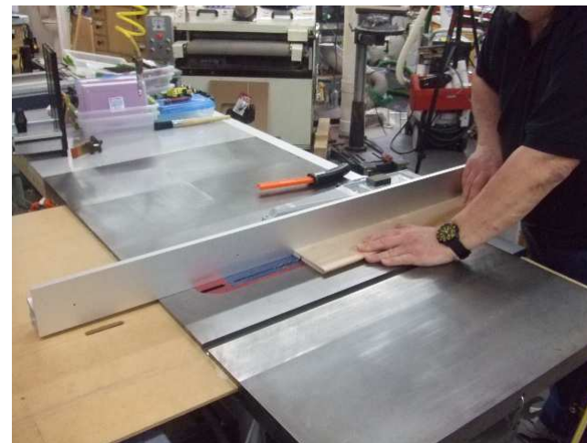
\frac{1}{8} " or \frac{1}{4} " dado, \frac{1}{4} " deep, \frac{7}{8} " from edge - table saw
