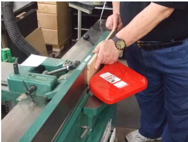
\frac{1}{4} " x \frac{1}{4} " rabbit on top edge - jointer, router, table saw
