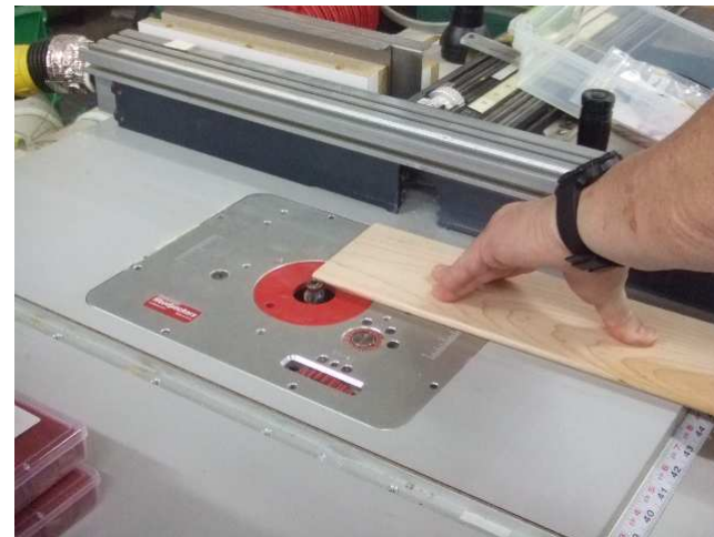
\frac{1}{8} " round-over outside of top edge - router
