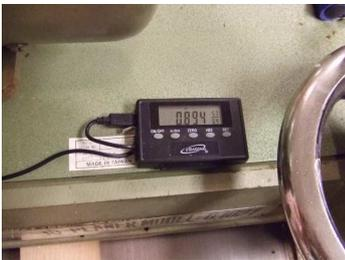
readout when needed. The display unit has a pair of rare earth magnets, so you can place it in any convenient
