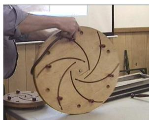
don't fit some bowl sizes. They found diagrams for a homemade Longworth chuck that uses a scrolling action to provide an infinite
