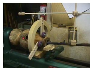
They also made wall thickness indicators that use a laser to measure the thickness of the wall as they are hollowing out the interior of the vessel.
