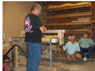
John Phelps did the electrical work, as well as the computer system and interface design and installation. Jerry's son-in-law, John Bourgeois, uses computer graphics software to translate the desired design into machine code that drives the router to carve the wood. So far, they've made some signs and carved various logos into blanket chests and tables.
