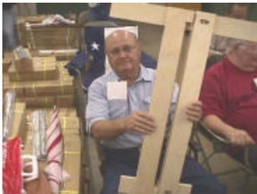
Dale Clark made this jig to cut perfect dados. It's adjusted to the thickness of the material after it's sanded.
