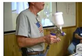
The cans can either be on top (gravity feed) or the bottom (siphon feed). Waid, and most automotive painters,
