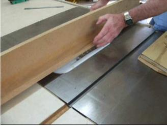
The runner is positioned about  $7/8$ " above and exactly in line with the table saw blade.
