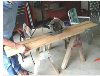
Nail a straight, narrow board to a piece of plywood that's longer than the cut you have to make. Then run your saw along the
