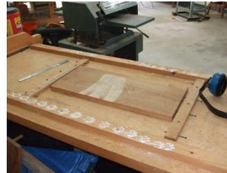
It consists of a large flat surface (George used a solid core door) with runners that are thicker than the panel and
