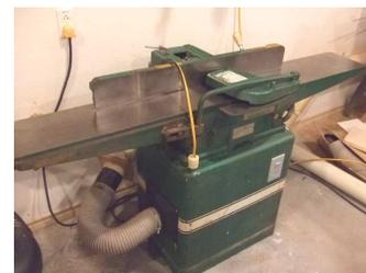
After replacing the drive pulley and installing a new belt, he made a test cut and the jointer performed perfectly.
