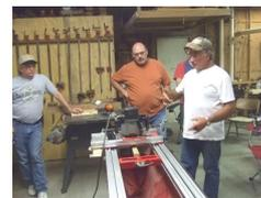
Jerry explained the operation of the machine as he demonstrated it. He took a square piece of wood and worked it first into an octagonal shape then a cylindrical shape, and then he worked decorative grooves into it.
