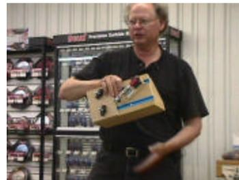
Gary Moffatt built a special jig to rout the ends of the rails on his raised panel doors.
