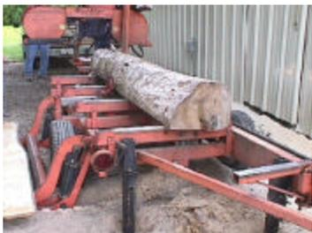
lumber yield from the log. Since the Wood-Mizer is a band saw mill, there is minimum kerf waste.
