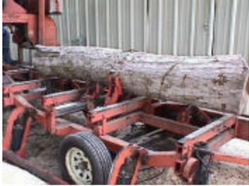
diameter. It can cut boards as wide as 28" in one pass. It has a 24 HP gasoline engine that powers the blade, the
