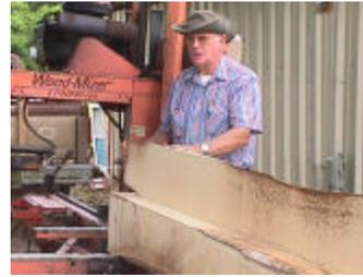
After the boards are cut, the edges are trimmed to remove the bark and square them up. Bill stacks the boards on edge,
