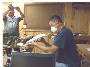
Rob Emanuel presented a program about sanding, gluing and assembling an intarsia picture. Rob does most of his shaping using sanding drums with foam cores. The foam is soft enough not to gouge the wood pieces and produces smooth contours. They're available from Seyco Scroll Saw
