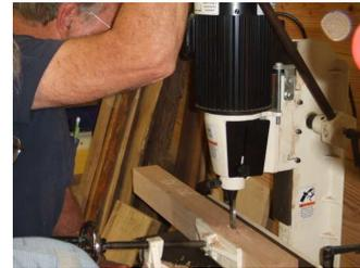
best display the grain. Then they marked and cut the mortises using Steve's mortising machine. They also used a hand-held
