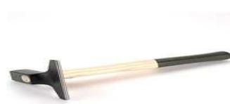
hammer and saw. The veneer hammer is not truly a hammer, a blunt, rounded edge blade
