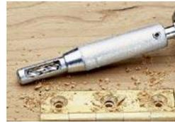
aligns the doors and mounts the hinges. He also uses a VIX bit to center the pilot holes in the hinge. Waid also
