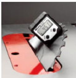
Richard Hicks and Steve Brady both brought one of the new Wixey electronic angle gauges. It can be used to measure and set the angle on any power tool. You set the tool on
