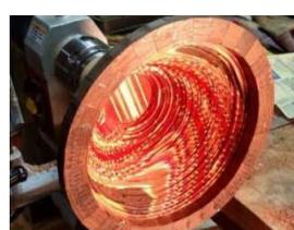
Then select, dimension and glue the various species of wood together. Then resaw the blank into smaller blanks and layout the rings. Then cut and label the rings so they can be assembled in the proper order. Mark glues two rings together so they won't be as fragile to handle. It also speeds up the subsequent gluing steps. He dry fits the rings and marks their relative location. It's important that the offset from ring to ring be consistent so the "dizzy" pattern develops correctly.
