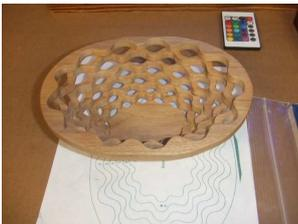
It starts as a flat board and as each ring is cut, it's rotated 90 degrees and glued to the previous ring to form a basket.
