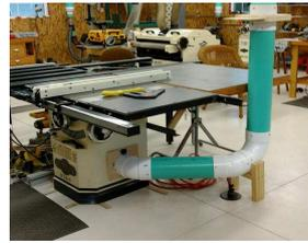
Ronnie Webb showed pictures of the completed installation of his 6" dust collection system going to his table saw and jointer. Ronnie had to fabricate special ports for the tools to accommodate the 6" pipe connections.
