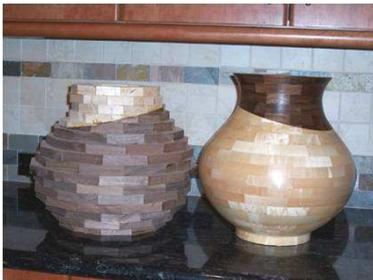
many pieces of wood together to make a blank that is turned on a lathe to make vase or bowl.
