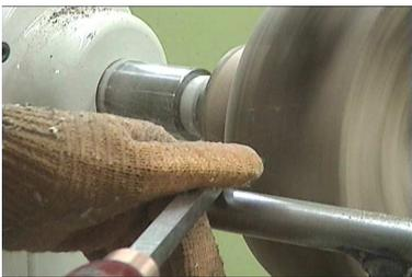
Start the lathe at the slowest speed in case the blank isn't balanced. Establish the outside profile
