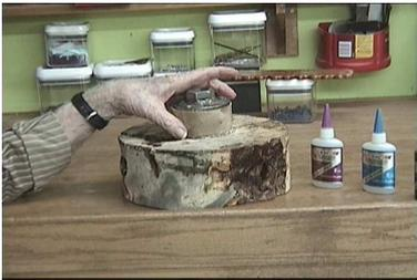
The first step is to get the blank ready to turn by cutting it round on a band saw and gluing a waste
