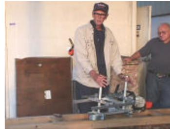
an inexpensive alternative to a larger mill if you just have a small number of logs to mill. It has a holding mechanism for the motor end of the chainsaw, a tracking bar and another attachment for the end of the chain bar. You can
