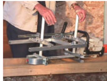
use almost any brand and size chainsaw and you have to use a 'ripping' chainsaw blade.
