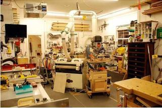
His shop layout groups equipment and supplies together based on the way they are normally used. For example, his turning tools, lathes and supplies are in one location. His material preparation area includes his jointer, planer and table saw. His frequently used items are also in plain view and easy to get to.
