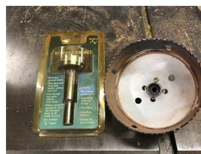
To make the washers, Jim takes a thick hole-saw and uses a 3 1/2" hole-saw to cut a round blank and uses a 1 5/8" forstner bit to
