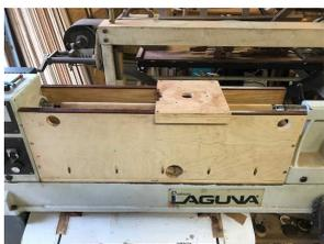
between centers on his lathe and uses a router with a 'bottom cutting' bit, riding on a homemade track, to machine and sand the dowels to 1 1/2" +/- .005" which is critical when cutting the threads. He cuts the dowels to about 6" long.
