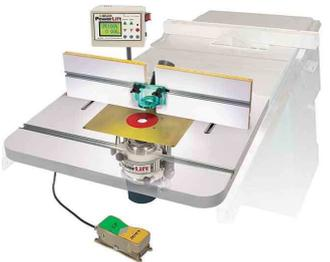
David built his cabinet to house his new MLCS Powerlift Motorized Router Lift. The lift uses an electric motor to raise and lower the
