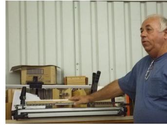
about making dovetails with a Leigh Jig. The Leigh jig is very flexible and makes through or half blind dovetails.
