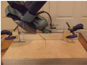
This is the jig he uses on his compound miter saw for cutting the miters on small boxes. The blade is tilted 45 degrees and the
