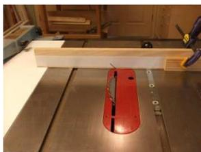
This is the miter gauge setup he uses when cutting larger boxes. He likes to use  $\frac{3}{4}$ " plywood scraps (as long as they are flat)
