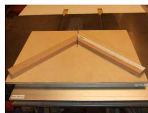
This is the sled that he uses for cutting the miters on picture frames. He described the steps in making the sled so that it fits your saw and cuts accurate miter joints. The
