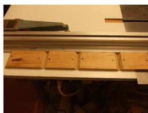
Richard usually uses his Unifence to align the box parts prior to applying glue to the miter joints and he usually uses packing
