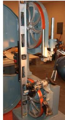
A 'co-planer' wheel adjustment should be performed at least once on every bandsaw - even brand new ones. This involves using a straight edge to ensure the wheels are aligned with each other. If they aren't aligned, adjust the alignment by adding
