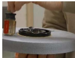
and he recommends using the OSHA 'ring test' that specifies supporting the wheel on your fingertips and tapping the wheel with
