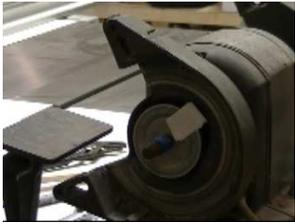
adhesive dots or labels between the wheel and the inboard mounting washer opposite the apex of the arc.
