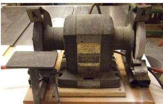
lathe chisels but it vibrates so badly that he doesn't like to use it. An article by Don Geiger in the December Issue of the American Woodturner detailed a procedure for mounting and truing the wheels to eliminate the vibration.
