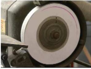
Start the grinder and lightly touch the marker to the surface.
