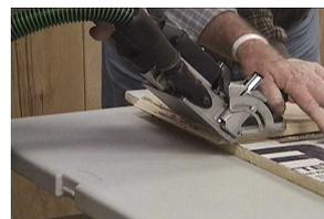
Then he used the Festool Domino joining system to install 'tenons' in the 45-degree angle joint.
