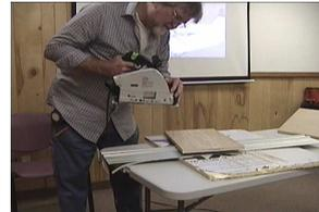
degree angle using the Festool plunge saw and track system. He noted that the saw cuts exactly on the edge of the guide
