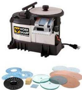
The Work Sharp system uses sandpaper on a glass wheel to sharpen various shop tools. Grits are available from 120 to 3600. It also has a unique see-
