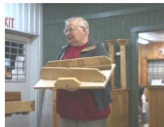
This is a jig he uses to cut LARGE SIZE dovetails in things like cabinets and chests. And this is a special jig used to cut tenons on his router table.
