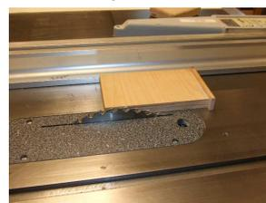
cut multiple pieces of wood 5/16" thick for a toy project, he built a jig based on the tip. He cut a scrap piece of plywood 4" wide and attached a short strip of wood to the edge
