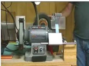
Rob uses a slow speed grinder (~1,800 rpm) with a 120 grit wheel. He uses a Tormek jig on his grinder. He starts by flattening
