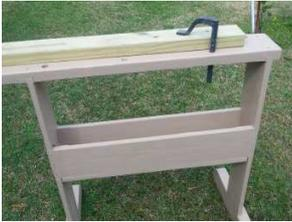
Tommy Ellis showed a picture of a work bench he made. It's build like a saw horse and uses bench hold down clamps to hold the workpiece.
