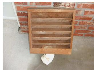
Richard Hicks brought a home made dust collector attachment designed for a radial arm or miter saw.
