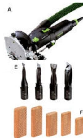
B.J., (Woodworker's Paradise), brought a Festool Domino Joiner. The tool uses a patented mortising technique designed to accept special "domino" tenons. Special cutters, along with very precise indexing fences, assure a perfectly fitting joint every time. The
