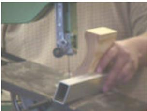
John cuts the profile on a bandsaw and also uses a bandsaw to remove excess material before he does the final
