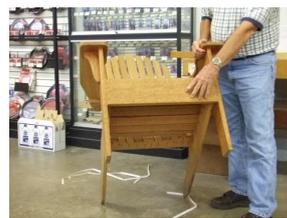
Dean uses a lot of templates to rout the various shapes. The chair must be assembled in a particular order for all the pieces to fit properly. He provided a material and cut list along with detailed instructions. He suggests that you precut all
