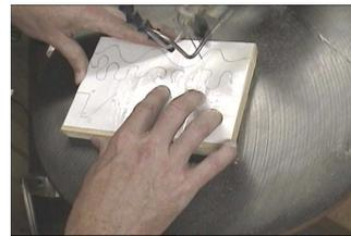
cutting the project. He adds a layer of packing tape to the top of the pattern to lubricate the blade while making the cuts.
