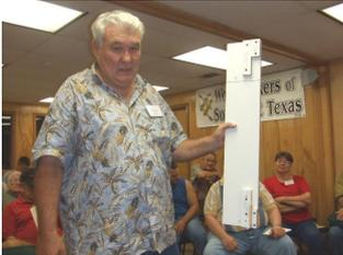
Tommy Ellis made a jig to cut tapered legs for a table project he's working on.
