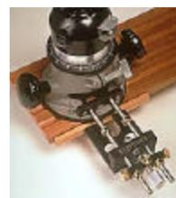
John Phelps showed us the MicroFence adjustable fence router accessory. It's custom made for each brand and model of router and it adjusts to an accuracy of
