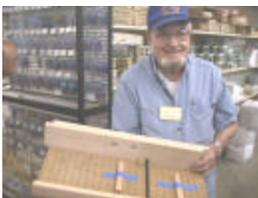
Howard Hartman showed us a box joint jig he uses with his table saw. He also brought an example of a box joint he made with his jig to prove it works.
