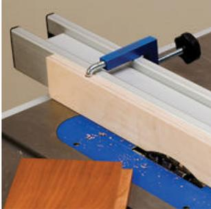
existing fences without having the clamp interfere with your work. The clamp arm simply fits into a 3/8" hole in the top of the auxiliary fence, keeping it out
